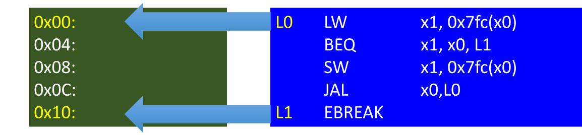
The label "L0" is a symbolic name for the memory location with address 0x00. Likewise, the label "L1" is a symbolic name for the memory location with address 0x10.
